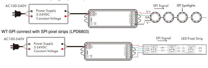
WiFi-SPI connects with SPI digital light tube (TM1809)
