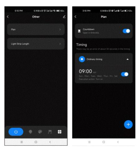
• Countdown: Customize the countdown time (Max.24 hours) to perform the on/off action. Timer: Customize multiple times (days of the week) to perform the on/off light action.
