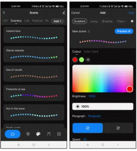
44 predefined scenarios and 10+ custom dynamic scenarios selectable. The custom scenarios can select 16 types variations (fade, jump, breath, flash, flow, rainbow, shooting star, pile-up, floating down, chasing light, floating, flashing, bouncing, shuttle, chaotic flashing, open and close), the 1-8 colors, full or segment control, forward or reverse motion direction, adjustable brightness and speed.
