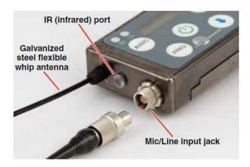
The antenna is a flexible whip made of galvanized steel, permanently attached to the transmitter to prevent damage from heavy use. The IR port is capped with
