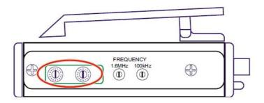
On older transmitter models, the left hand switch makes steps in 1.6 MHz increments, the right hand switch in 100 kHz increments. Each block spans a 25.6 MHz band. A simple formula is used to name the blocks according to the lowest frequency in each one. For example, the block starting at 512 MHz is named Block 20, since 25.6 times 20 equals 512.
