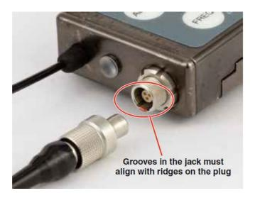
Slide the threaded sleeve onto the jack and rotate it clockwise to tighten it.
