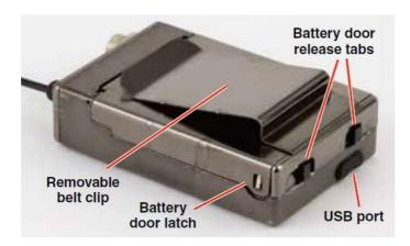
The battery door itself is made of stainless steel to allow a thin wall thickness, but retain the strength to withstand heavy use.
