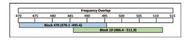
Frequencies 486.400 495.600 Overlap in Blocks 470 and 19. Block 470 and block 19 overlap each other in the frequency range from 486.400 to 495.600 MHz. Since block 470 starts at a lower frequency than block 19, the hex codes and pilot tones will not match even though the frequencies are the same in the overlap zone. When using a transmitter on the A1 band with a block 19 receiver be sure the transmitter is set to block 19 and check the hex
