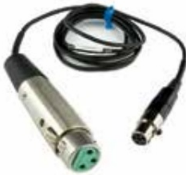
MC41 mic level adapter cable. Female XLR to female TA5F; 37 inches long. Feeds mic level signal to pin 3 on the TA5M jack.
