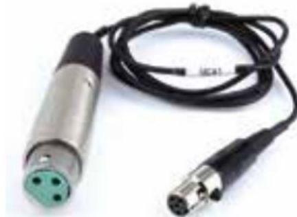
MCAES3 Used to connect the output to the AES3 digital input of a mixer or recorder; TA5F jack to 3-pin female XLR connector
