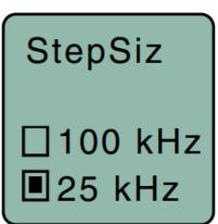
If the desired frequency ends in .025, .050 or .075 MHz, the 25 kHz step size must be selected.
