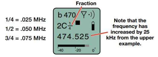
Changing the step size never changes the frequency. It only changes the way the user interface works. If the frequency is set to a fractional increment between even 100 kHz steps and the step size is changed to 100 kHz, the hex code will be replaced by two asterisks on the main screen and the frequency screen.
