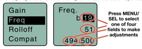
Each field will step through the available frequencies in a different increment. The increments are also different in the 25 kHz mode from the 100 kHz mode.
