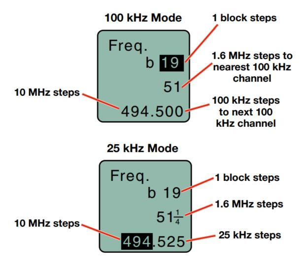
If the Step Size is 25 kHz with the frequency set between even 100 kHz steps and the Step Size is then changed to 100 kHz, the mismatch will cause the hex code to display as two asterisks.
