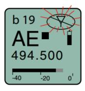
To enable the RF output from the Standby Mode, press the Power Button, select Rf On? option, then select yes.
