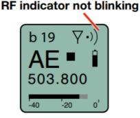
If the button is released before the countdown is completed, the unit will power up with the RF output turned off.
