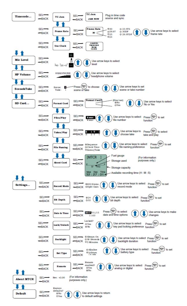
When TC Jam is selected, JAM NOW will flash on the LCD and the unit is ready to be synced with the timecode source. Connect the timecode source and the sync will take place automatically. When the sync is successful, a message will be displayed to confirm the operation.
