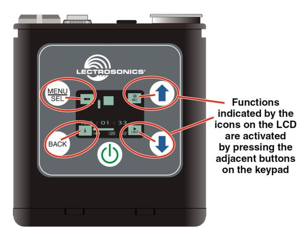
Icons in each corner of the LCD define the alternate functions of the adja-cent buttons on the keypad. For example, in the Main Window shown above, recording is started by pressing the UP arrow button on the keypad, in which case, the display switches to the Recording Window.
