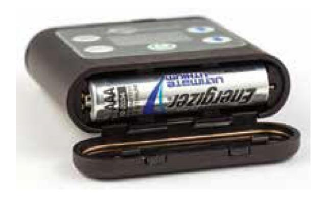
**CAUTION:** Danger of explosion if battery is incorrectly replaced. Replace only with the same or equivalent type.
