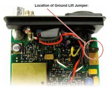
Jumper placed toward PCB as shown connects pln 1 to ground. Move Jumper to outside contacts to lift ground.
