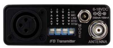
**XLR Jack** A standard XLR female jack accepts a variety of input sources depending on the setting of the rear panel MODE switches. XLR pin functions can be changed to suit the source depending on the positions of the indi-vidual switches. For detailed information on the setting of these switches see the Installation and Operation section.
