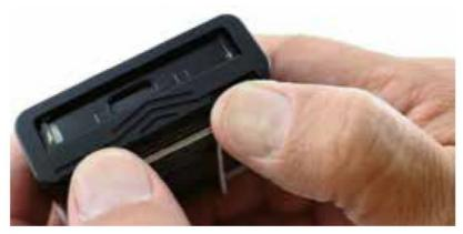
Slide the battery compartment door open, drop the battery in so that the connectors match, and slide the battery door closed. The battery door will now "lock" when fully closed. To "unlock," press down the actuator and slide the battery door open.
