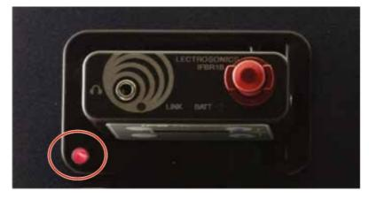
When a battery or IFBR1B is being charged the LED next to it will glow RED. When the battery is fully charged, the LED will glow GREEN. If a fault occurs, the power to the slot will be disabled and the LED will turn off.
