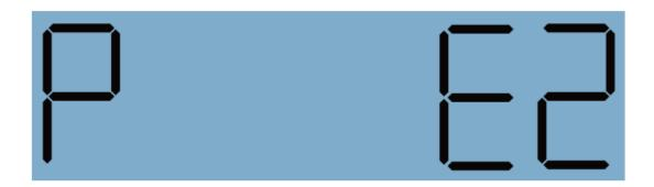
If the current preset slot is empty, an E also appears on the right. Use the UP and DOWN arrow buttons to navigate among any programmed presets, tuning the receiver to each.
