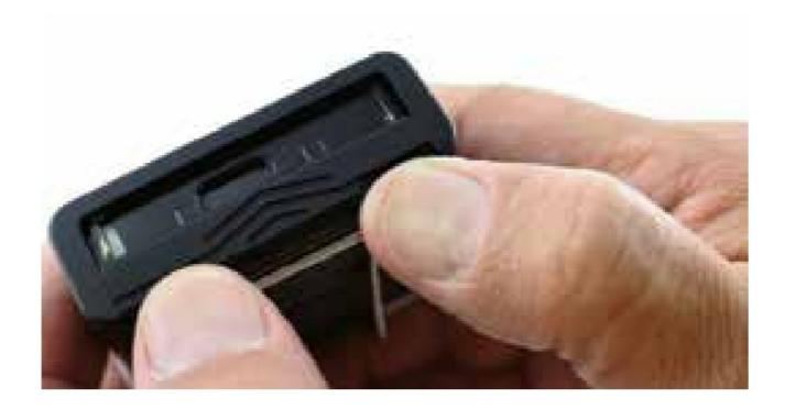
Slide the battery compartment door open, drop the battery in so that the connectors match and slide the battery door closed.
