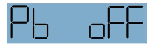
The setting page is labeled "Pb." The default value is OFF. Pressing the DOWN button changes the value to ON, while pressing the UP button will change the value back to OFF.
