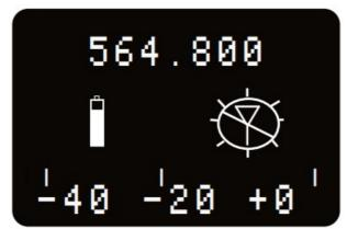
In this Standby Mode the frequency can be browsed to make adjustments without the risk of interfering with other wireless systems nearby.
