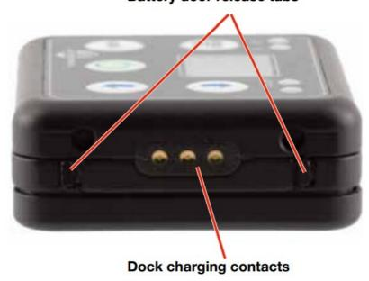
The opposite end of the transmitter contains the battery door latches and release tabs, along with the dock charging contacts.
