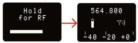
When you release the button, the unit will be operational with the RF output turned on and the Main Window displayed.
