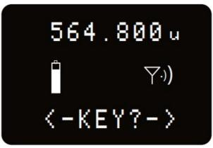
The DSSM ships with the key type set as "Universal" and will work right away with any receiver also set to Universal Key Type.
