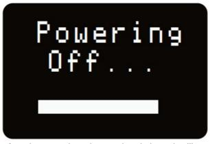
If the power button is released before the countdown is completed, the unit will remain turned on and the LCD will return to the same screen or menu that was displayed previously.
