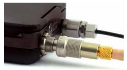
Slide the threaded sleeve onto the jack and rotate it clockwise to tighten it.
