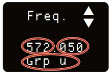
Press MENU/SEL and use the arrow buttons to select one of three fields to adjust: MHz, KHz and Group.
