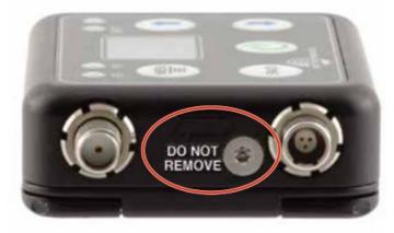
CAUTION: DO NOT REMOVE the threaded screw where indicated, as that will void the warranty and IP rating.
