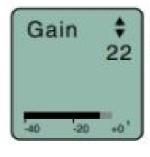
Use the UP and DOWN arrow buttons to adjust the gain until the -20 LED blinks red on louder peaks
