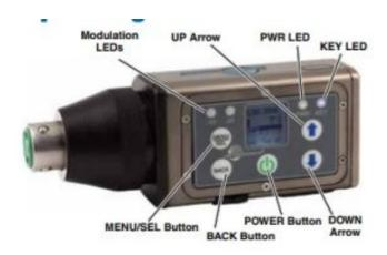
To format the card with the DPR, select Format Card in the menu and press **MENU/SEL** on the keypad. NOTE: An error message will appear if samples are lost due to a poor performing "slow" card.WARNING: Do not perform a low level format (com- plete format) with a computer. Doing so may render the memory card unusable with the DPR recorder.
