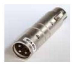
This adapter may be needed if you are experiencing noise or distortion with measurement microphones, particularly the Earthworks M30. The adapter has a common mode choke for suppressing RF noise. If your microphone signal exhibits the problems listed above when connected to a UH400, HM or DPR transmitter, insert the adapter between the microphone and the transmitter. Mic adapter for Earthworks M30 microphone with HM, DPR and UH400a/TM transmitters.
