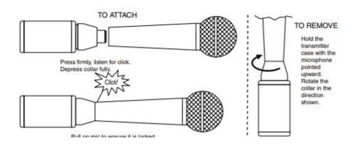
**NOTE:** Do not hold or apply any pressure to the microphone body while trying to remove it, as this may prevent the latch from releasing.
