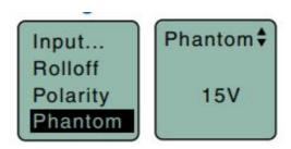
The transmitter input jack can provide phantom power for the attached microphone if needed, with voltages at 5, 15 or 48. Phantom power will consume a slight amount of battery power, so it can also be turned off.
