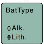
If you are using rechargeable batteries, it is better to use the timer func-tion on the receiver to monitor the battery life rather than the indicators on the transmitter. Rechargeable batteries maintain a fairly constant voltage across the operating time on each charge and stop working abruptly, so you will have little or no warning as they reach the end of operation.
