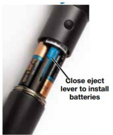
To insert batteries, close the eject lever and insert the upper contacts first (closest to the mic capsule). Polarity is marked on the label in the bottom of the battery compartment.
