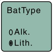
If you are using rechargeable batteries, it is better to use the timer function on the receiver to monitor the battery life rather than the indicators on the transmitter. Rechargeable batteries maintain a fairly constant voltage across the operating time on each charge and stop working abruptly, so you will have little or no warning as they reach the end of operation.
