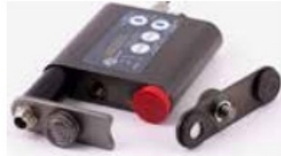
External power adapter (battery eliminator) for all SM Series transmitters. 6 to 36 volt external sources. Handles up to 1 amp consumption. Protected against shorts and reverse polarity.
