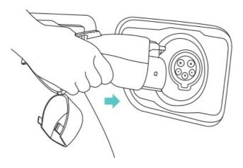
**Note:** The adapter must be plugged in within 1 minute of opening the charger door. Once it's plugged in, the adapter will automatically lock to prevent theft.
