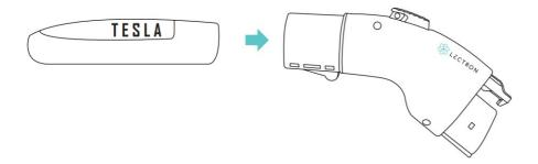
**Step1:** Connect the Tesla Charger to the Lectron Adapter. Wait at least 30s before connecting it to your J1772 electric vehicle.
