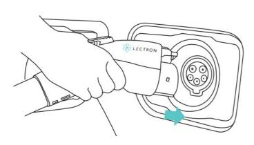
Step 2: Firmly plug in the Lectron Adapter into your J1772 electric vehicle.
