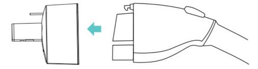
3. Insert the adapter into the Tesla charge port and wait for the vehicle to signal that it has accepted the charger with a pulsating green "T" light next to the charge port (the touchscreen also shows the real-time charging status).
