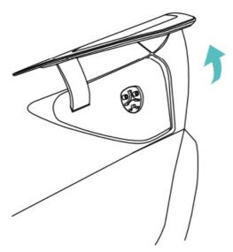
2. Insert the CCS1 charging cable into the CCS1 port on the adapter. It will click firmly in place.
