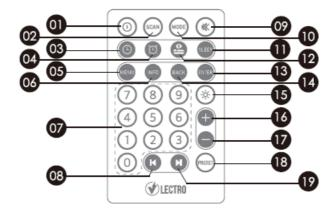
Use a CR2025 3V battery for remote control1 positive side facing up. Please take out the insulation tab plastic before using it!
