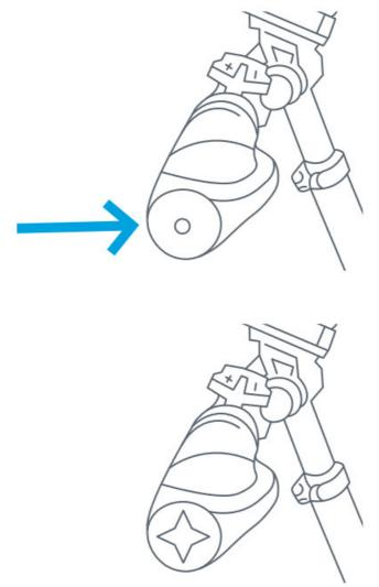
To begin, you will need to create a larger opening at the end of the rubber handlebar grip. (Behind your handlebar grip, your handlebars are hollow, this is where the collar of the mirror will fit into). Use a knife to create a larger opening for the mirror collar.
