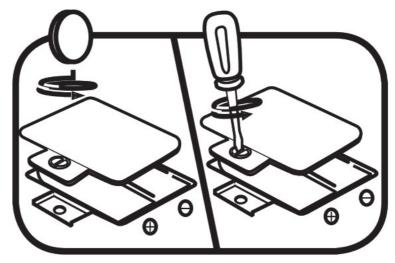
5. Replace the battery cover and tighten the screw to secure.
