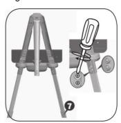
15. Fit Lower Rear Leg into the top of A-Frame 1/2 with the curved side of the leg facing up. Secure with two Nuts and two Bolts, inserting the Nuts from the top.
