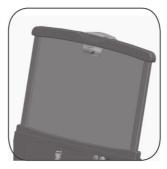
19. Slide the Board Clip Release switch to the right and while holding it, lift the Board Clip.
