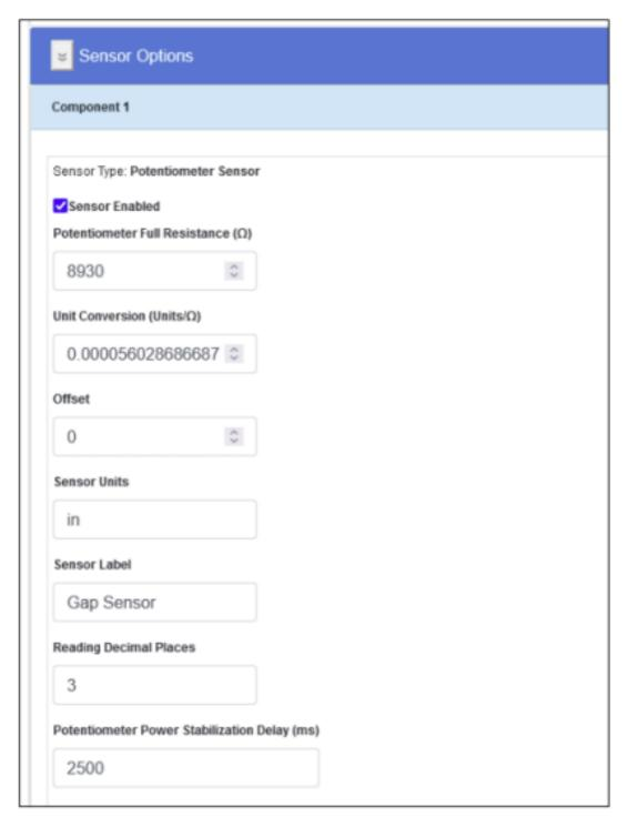
If Phase IV sent the **Leap Linear Potentiometer Sensor Device** with a Linear Potentiometer Sensor already connected it will already be configured and calibrated. Adjusting the configuration won't be necessary. If connecting a Linear Potentiometer Sensor in the field adjust the options as appropriate as described below:
