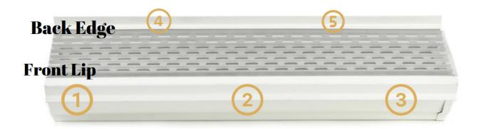
The tab on the left end of each panel installs under the adjoining panel. Use screw holes along the front lip of Leaf4go Micromesh to zip screw the panel – 3 or 4 screws (1, 2 & 3) to the front lip of the gutter and 2 screws for the back (4 & 5). DIAGRAM 2: Shows recommended cuts for connecting inside corner pieces together.
