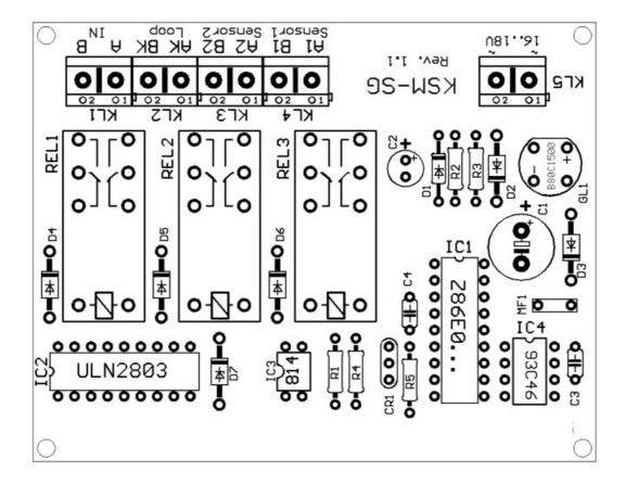
The input A and B of the reverse-loop module KSM-SG will receive the digital current from the command station or from a booster from the ring-conductor "driving". It is important that the reverse-loop will be complete inside one booster area and not between two rail sections which get the supply from two different boosters.
