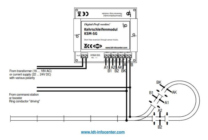
Sample Connection 2: Reverse-loop polarity via the reverse-loop module KSM-SG plus track occupancy report at the reverse-loop with the RM-GB-8-N. Sensor tracks will be monitored as well.
