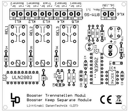
The Booster Keep Separation Module BTM-SG provides a secure electrical separation between the booster current circuits.
