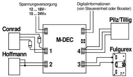
The above draft provides an example how to connect the different drives directly to the M-DEC-DC without any additional circuitry.
