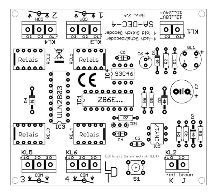
Remarks: The decoder addresses for magnet accessories are combined in groups of four. The address 1 to 4 build the first group. The address 5 to 8 build the second group etc.
