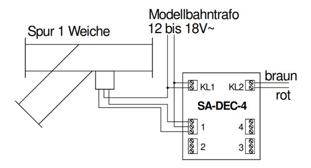
Feed the SA-DEC-4 via clamp KL1 witch AC from the model railway transformer. Further, connect one ac-cable of the transformer with clamp 'L' on the turnout drive. Connect the second cable of the transformer with the clamp marked 'COM' on the respective decoder output.
