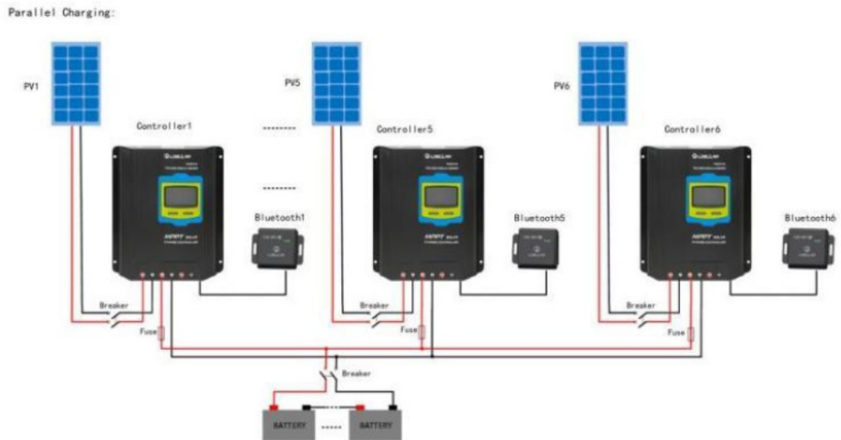
Figure 2-2 Schematic of wiring diagram
