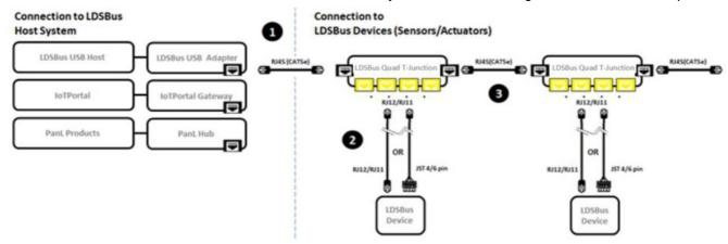
Note: Enable termination for last LDSBus Device in the bus
