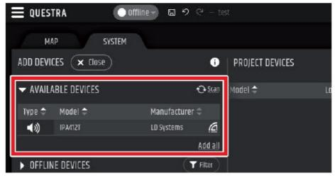
Drag and drop the device into the PROJECT DEVICES area to be able to configure it. Then click the Offline button at the top of the screen and select Download from Devices and connect to the device.
