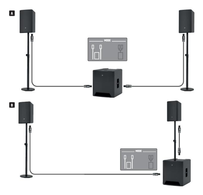
If the standard set-up of the DAVE G4X speaker system is not desired or possible, the set-up can be done with a distance rod and a stand fork mounted on the subwoofer C . In order to achieve an impressive stereo sound and to avoid unpleasant interference, select the DSP preset that corresponds to this setup variant (MODE SELECT, right symbol) and use the stereo input INPUT 3L / 4R for control (XLR/jack combo sockets or cinch sockets).
