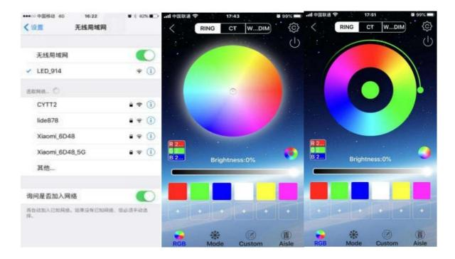
When the connection is successful, open the LED LAMP application software, and the color circle control interface will appear, and the corresponding mode operation can be carried out at this time.
