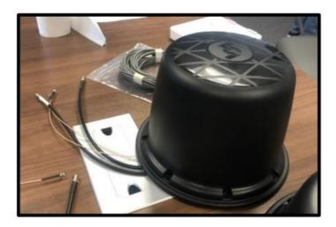
**Step 1:** Locate the area on the roof where the Antenna will be placed. The placement must make wiring accessible from the interior of the RV.
