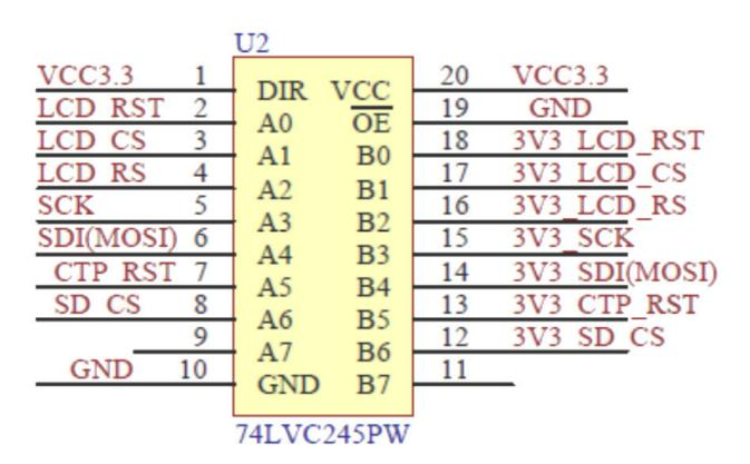
U2is a level conversion IC that converts between 5V and 3.3V. This circuit only uses the one-way function of 5V to 3.3V, and the signals that the module needs to write are converted through this circuit.
