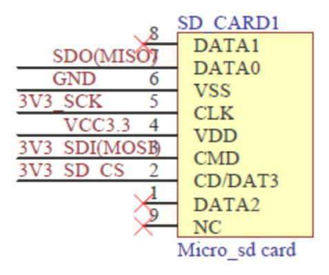
SD\_ CARD1 is a Micro SD card slot for inserting Micro SD cards, making it easy to use SD card expansion functions. The SPI bus and LCD used are shared.
