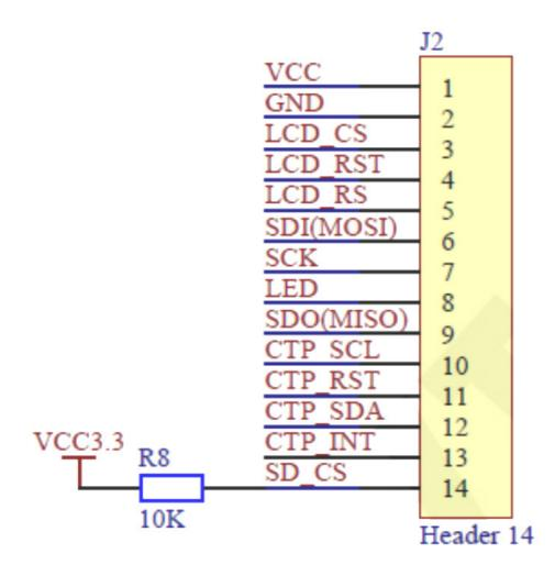
J2is 14P pin, R8 is the pull-up resistor of SD card CS pin. The 14P pin is used to connect to the main control, which can be directly inserted or connected through a DuPont cable. Because the SD card and LCD share the SPI bus, first pull up the CS pin of the SD card to disable its functions and avoid SPI bus device conflicts when the module is in use.
