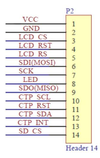
P2 is the module 14P FPC cable interface, which can only be connected to the main control through the FPC cable.
