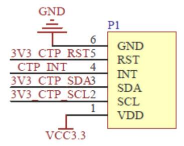
P1is a flip over FPC holder with a spacing of 6P 0.5mm, used to connect the 6P FPC cable of the capacitive touch screen and connect touch signals.
