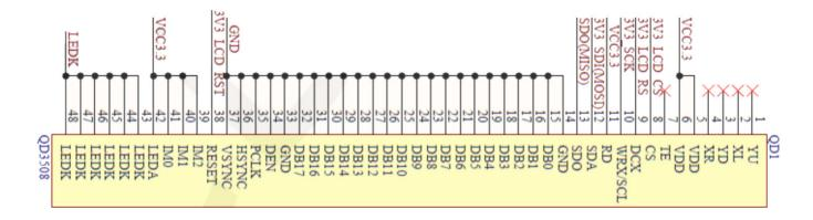
QD1 is a 48P pad with a spacing of 0.8mm. Used to weld the LCD so that it can receive signals from the main control.
