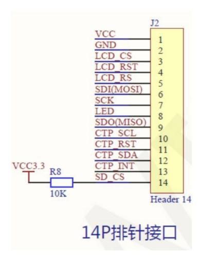
J2 is 14P pin, R8 is the pull-up resistor of SD card CS pin. The 14P pin is used to connect to the main control, which can be directly inserted or connected through a DuPont cable. Because the SD card and LCD share the SPI bus, first pull up the CS pin of the SD card to disable its functions and avoid SPI bus device conflicts when the module is in use.
