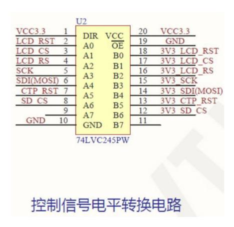
U2 is a level conversion IC that converts between 5V and 3.3V. This circuit only uses the one one-way function of 5V to 3.3V, and the signals that the module needs to write are converted through this circuit.
