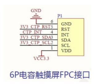
P1 is a flip over FPC holder with a spacing of 6P 0.5mm, used to connect the 6P FPC cable of the capacitive touch screen and connect touch signals.
