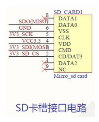
SD\_ CARD1 is a Micro SD card slot for inserting Micro SD cards, making it easy to use SD card expansion functions. The SPI bus and LCD used are shared.
