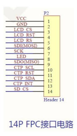
P2 is the module 14P FPC cable interface, which can only be connected to the main control through the FPC cable.
