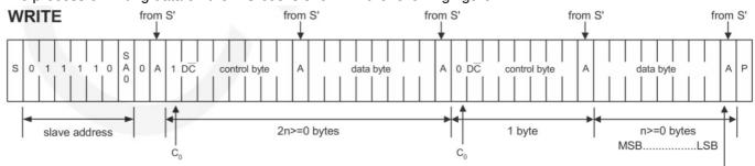
After the IIC bus starts working, it first sends the slave device address. After receiving a response from the slave device, it then sends a control byte to notify the slave device. The next data to be sent is a command to write to the IC register or data to write to RAM. After receiving a response from the slave device, it then sends
