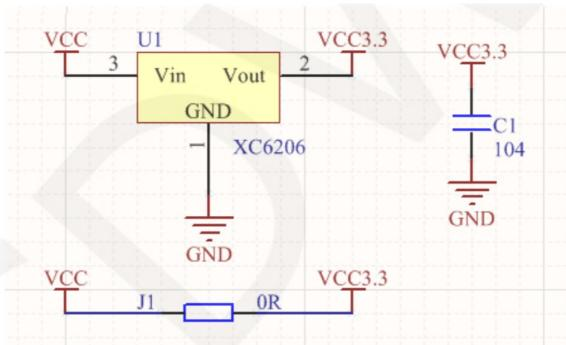
This circuit is a module system power regulator circuit, with U1 as the regulator, which can convert external input 5V or 3.3V voltage into 3.3V output, and C1 as the bypass filter capacitor.
