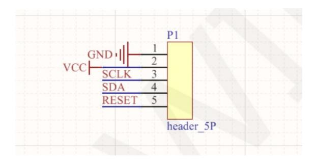
This is a 5P 2.54mm spacing row pin interface circuit used to connect to the main control. Among them, P1 is a 5P pin, and 1-5 pins are GND, VCC, SCL, SDA, and RESET respectively. Due to the internal reset circuit of the module, the RESET pin is not soldered by default. If you want to control the RESET function in the program, you need to solder the pin and connect it to the GPIO port.
