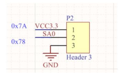
When selecting pull-up, select 0x7A slave device address; When selecting the dropdown, select 0x78 slave device address (default)
