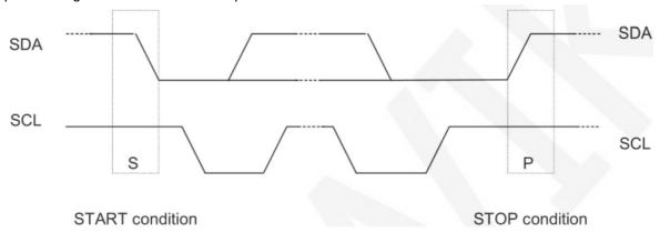
When both the data line and clock line of the [IC remain at high level, the IIC is in an idle state. At this time, the data line changes from high level to low level, and the clock line continues to remain at high level. The IIC bus starts data transmission. At that time, the clock line remained at high level, the data line changed from low level to high level, and the IIC bus stopped data transmission.
