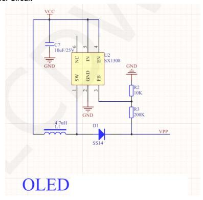
This circuitis an OLED external boost circuit, where U2 is an SX1308 boost IC.
