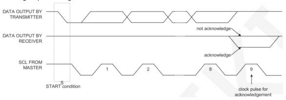
When the master device waits for the ACK from the slave device, it needs to keep the clock line at a high level, and when the slave device sends an ACK, it needs to keep the data line at a low level.
