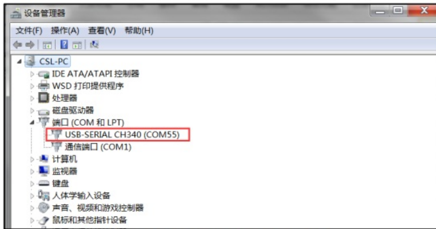
Figure 3 Identifying CH340 ports
