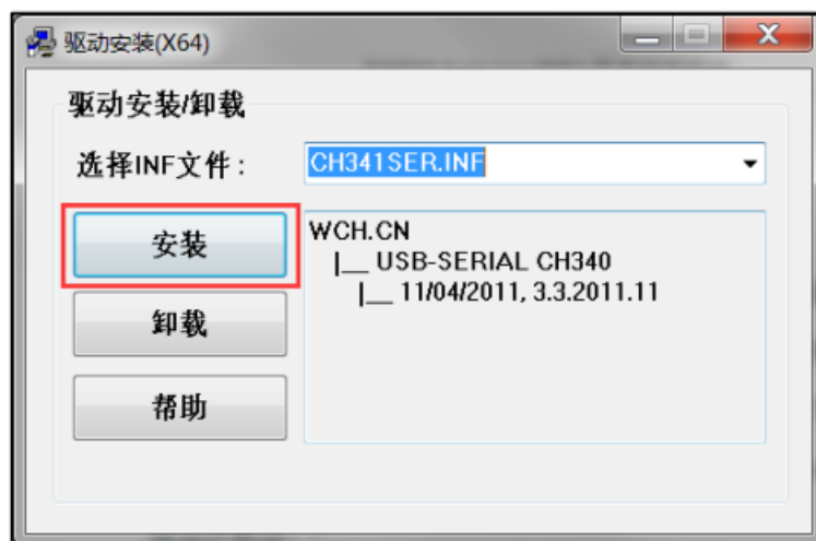
Figure 2 Installing the CH340C driver
