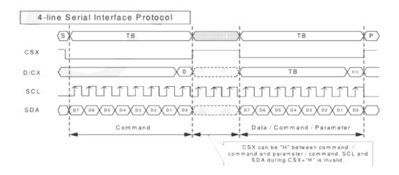
CSX is a slave chip selection, and the chip will only be enabled when CSX is at low power level. D/CX is the data/command control pin of the chip. When DCX is writing commands at low levels, data is written at high levels SCL is the SPI bus clock, with each rising edge transmitting 1 bit of data; SDA is the data transmitted by SPI, which transmits 8 bits of data at once. The data format is shown in the following figure:
