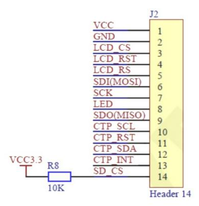
J2 is 14P pin, R8 is the pull-up resistor of SD card CS pin. The 14P pin is used to connect to the main control, which can be directly inserted or connected through a DuPont cable. Because the SD card and LCD share the SPI bus, first pull up the CS pin of the SD card to disable its functions and avoid SPI bus device conflicts when the module is in use.
