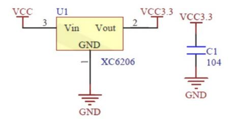
This circuit is used to stabilize the input voltage of the module, where VCC is the external input voltage, VCC3.3V is the module input voltage, and C1 is the bypass filter capacitor. VCC can be connected to 5V or 3.3V, and it is recommended to connect to 5V because only by connecting to 5V can VCC3.3 output 3.3V. If connected to 3.3V, VCC3.3 output voltage will be less than 3.3V, which will cause the backlight brightness of the LCD screen to darken.
