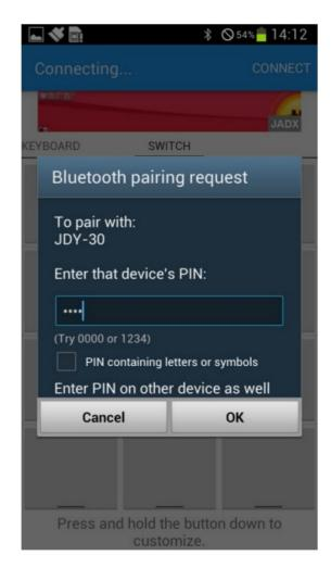
2. Install the "BlueSPP\_37" APP on your Android phone, enable your phone's bluetooth function. Open the APP and click "connect", select BLT device (such as BTA-04, JDY-30,etc) and insert password(the default password is 1234)
