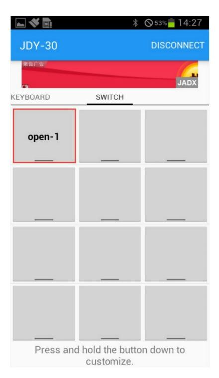
4. Finally you can send serial command to control the relay by click the function blocks.
