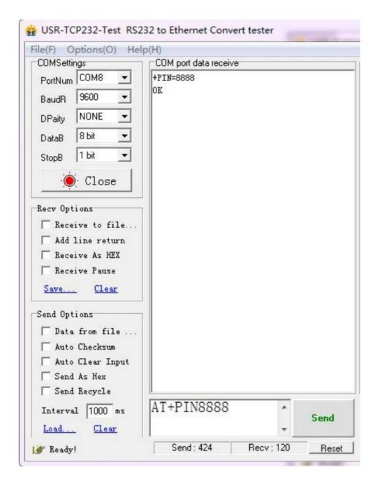
2. Modify the BLT name: For example, if we want to change the device name to LCTECH(default is BTA-04,JDY-30,etc), we can send "AT+NAMELCTECH", and then send "AT+RESET" can set the device name as LCTECH.
