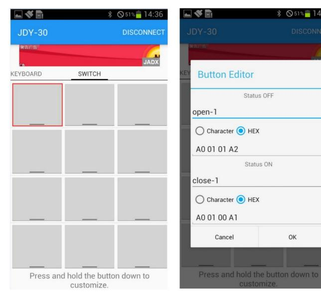
3. Press the function blocks and enter the name and content of the serial command (A00101A2 open relay, A00100A1 closed relay, command format must be hex)
