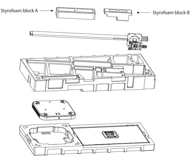
2. Place the stand base into the cavity of the upper styrofoam part and use the styrofoam block A to assemble the stand pillar as shown below:
