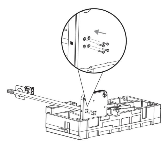
4. Hold up the stand, then assemble the display and the stand. You can use the display's "cavity slot" and the stand's "bracket hook" to hold up the display easily. Put the power socket at the "left side" position, then you can align the display close to the stand bracket until you hear a click sound.
