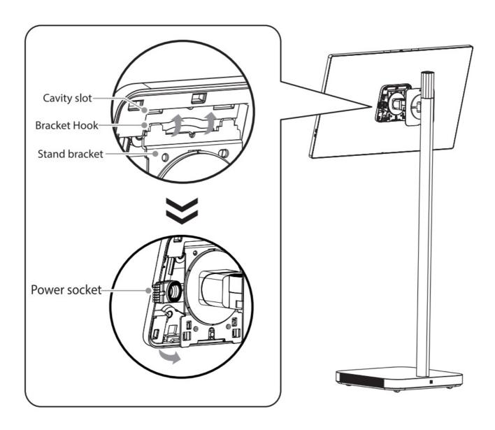
**Note:** Please make sure to have the power socket on the "left side" position before connecting the display and bracket.
