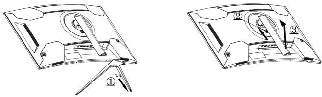
Remove the stem from the back side of the monitor (4).
