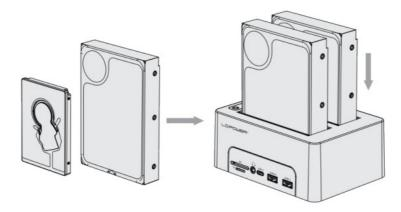
**1.2** Connect the power cable to the docking station and push the power switch on the back of the docking station. The computer will find the new hardware and install the matching USB driver automatically.
