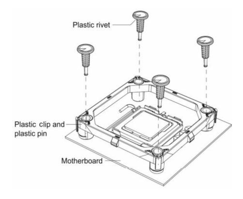
1. Put the CPU cooler to the center of the plastic clip. Hitch the tail of the cooler clip to the plastic clip. Then move the other side of the cooler clip and hitch it to the other side of the plastic clip.
