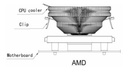
2. Connect the fan cable connector to the power socket on the mainboard where marked as "CPU FAN". Start your computer and check if everything works properly and if the CPU is properly cooled, then finish installation.
