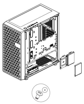
• Install SSD and secure with screws.
