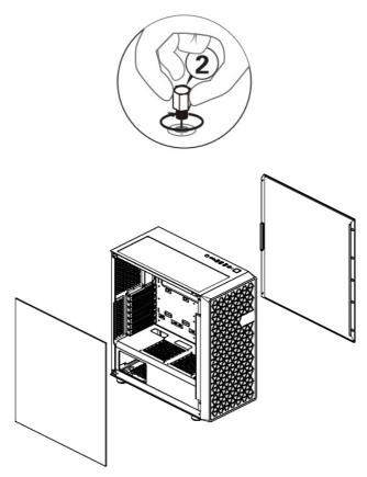
• Remove front and side panel retaining screws before attempting to remove either of the panels.
