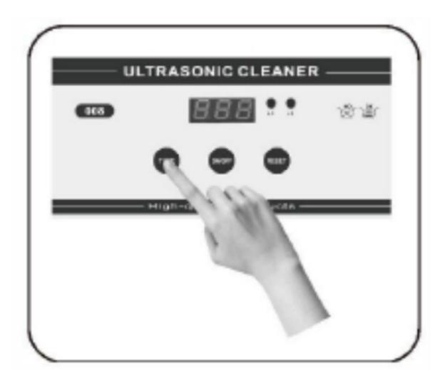
**Time Setting** Press TIMER multiple times in order to choose the amount of time you wish the items to be cleaned. There are 18 options: 90s 120s 150s 180s 210s 240s 540s 720s 900s 18m 21m 24m 27m and 30m.
