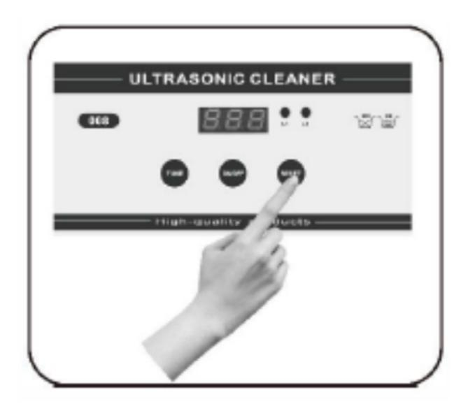
**Reset** Press RESET button when setting time or cleaning. Time will reset to "300" and machine will suspend work.
