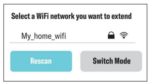
4. Enter the original password of the WiFi network that you want to extend (make sure to enter the exact password, otherwise the network will not be extended). Additionally, in this step, you can also set your own name for the network to be extended. Once entered, click the «Extend» button below.
