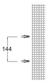
2. .Remove the product bracket, align it with the pre-made expansion rubber plug on the wall, lock the ST4.0 tapping screw, and fix the bracket on the wall.
