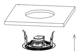
3. The product is clamped to the mounting plane by clamps.
