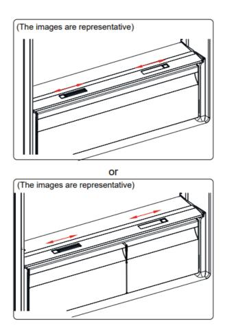
If the crisper is full, the fresh dial located in front of the crisper should be opened. This allows the air in the crisper and the humidity rate to be controlled, to increase the life of food within.
